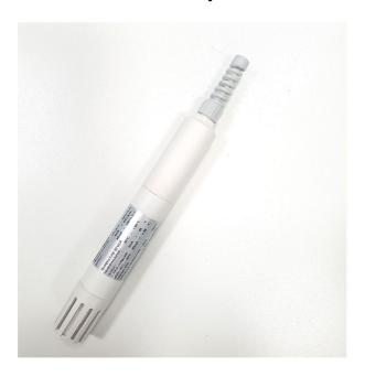
The TH1-M are single block RH and temperature microprocessor transmitters, temperature configurable. The TH1-MA is a passive transmitter with a 4...20mA output and 10...30Vdc power supply; the TH1-MV is a transmitter with a 0...1V standard voltage output and 5...35Vdc power supply. Sensors are mounted at the end of a plastic tube: a capacitive humidity sensor and a Platinum temperature sensor ( $100\Omega$  @0°C).
