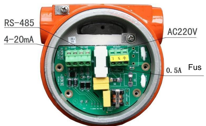
220VAC wiring terminal
